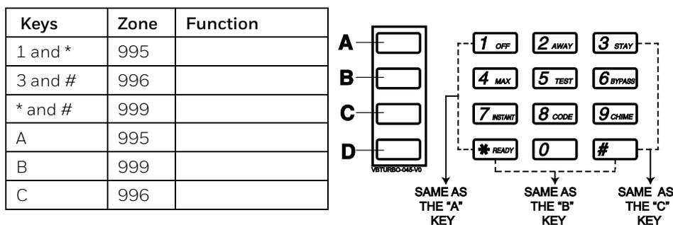
To use a paired key panic function, simply press both keys of the assigned pair at the same time.
